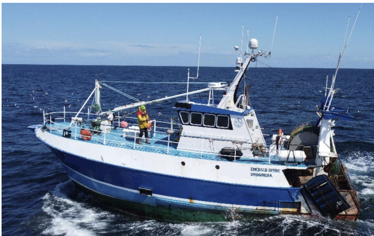
Figure 4.21 Example of demersal otter trawling vessel (Source: BIM, 2023)
