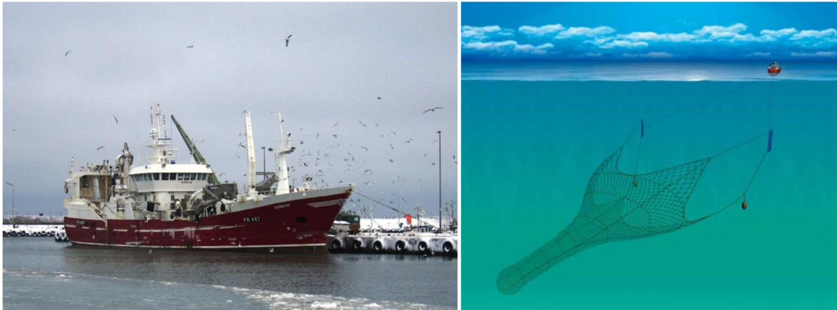
Figure 4.25 Typical pelagic trawling vessel and gear configuration (Source: Poseidon; and Seafish, 2015)
